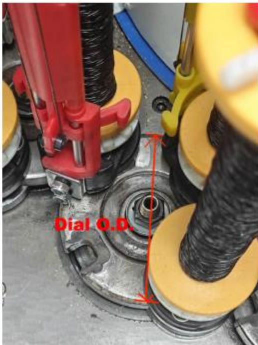
Larger Dial O.D., Larger Bobbin Capacity. You don't need to change the bobbin so often.
